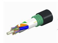
Fiber OSP cable, LazrSPEED® Single Jacket/Single Armor, Gel-Free, 72 fiber, Stranded Loose Tube, Multimode OM4, Feet jacket marking, Black jacket color
