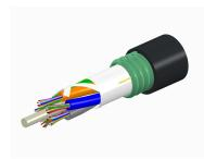
Fiber OSP cable, LazrSPEED® Single Jacket/Single Armor, Gel-Free, Stranded Loose Tube, 12 fibers, Multimode OM4, Feet jacket marking, Black jacket color
