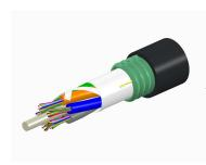
Fiber OSP cable, LazrSPEED® Single Jacket/Single Armor, 96 fiber, Gel-Free, Stranded Loose Tube, Multimode OM3, Feet jacket marking, Black jacket color
