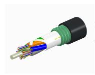
Fiber OSP cable, TeraSPEED® Single Jacket/Single Armor, Gel-Free, Stranded Loose Tube, 12 fibers, Singlemode G.652.D and G.657.A1, Feet jacket marking, Black jacket color
