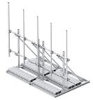
PIM-Guard High Capacity DUAL Non-Penetrating Roof Frame with Optimized Antenna Spacing 15 ft face, five 2-7/8 in OD x 120 in pipes
