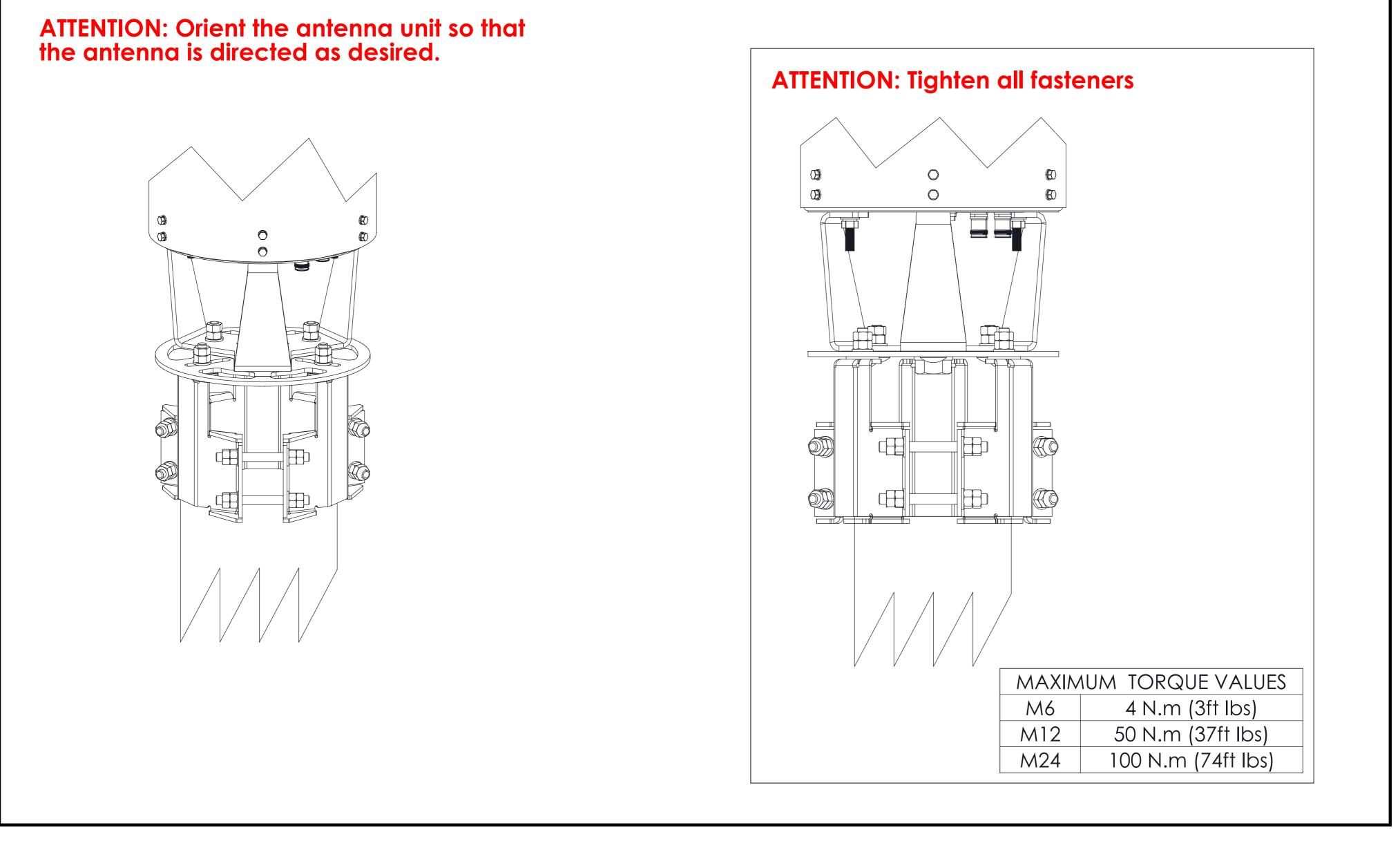
ORIENT ANTENNA AND TIGHTEN FASTENERS
