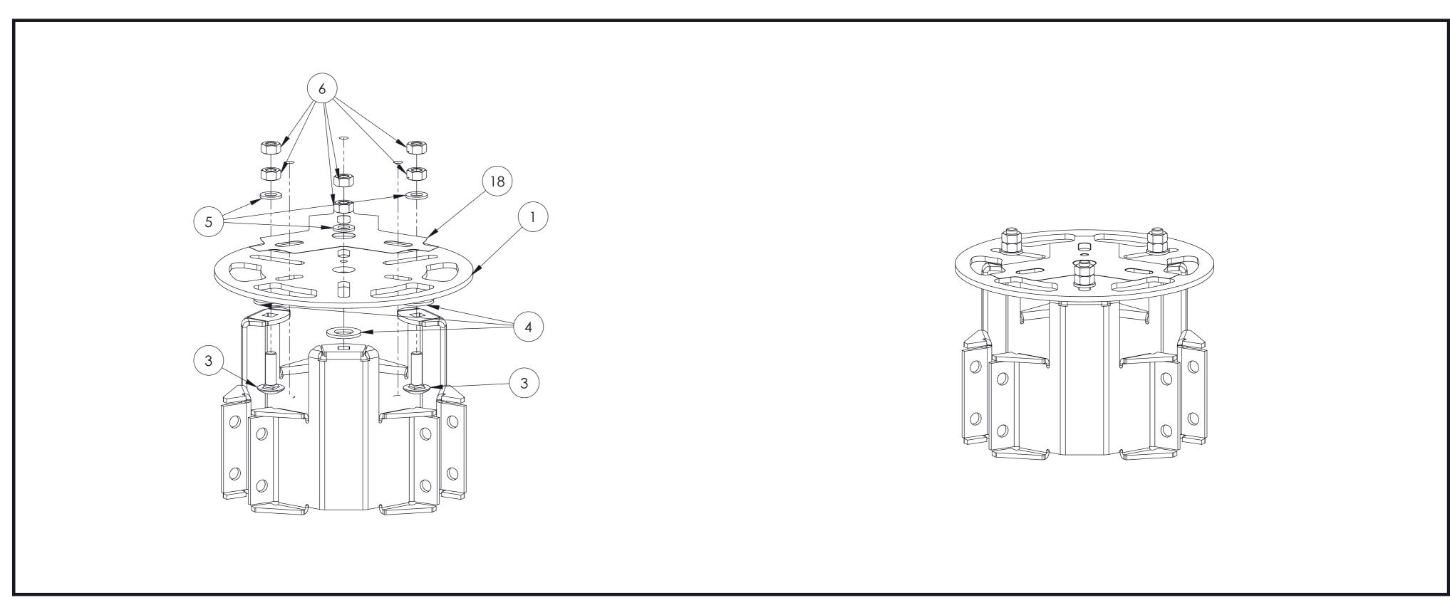
ASSEMBLE TOP MOUNT BRACKET TO PIPE MOUNT BRACKETS
