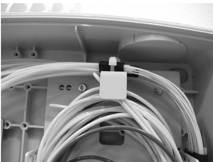
13.8. Two bundles of up to 12 tubes can be secured to the loop basket. When attaching the first bundle, make sure the second one can still be easily secured to the loop basket.
