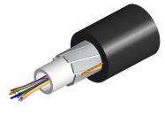
Fiber OSP cable, PE, Gel-filled Central Tube, All-dielectric, 12 fiber, Multimode OM5, Meters jacket marking, Black jacket color
