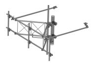
G23RHDXL PIM OPTIMIZED SPACING High Capacity Sector Frame with extended 10' Spine for RRU Mounting & extended frame for sites requiring increased sector to sector antenna spacing. 2 7/8in OD x 11ft face with (3) 2-7/8in OD x 126in Antenna pipes
