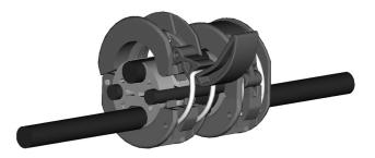
1.2.1 Install the 2 hinged clamps over each of the rubber sections of the branching plug; the raised ridge on the inside of the clamps fits into the groove in the rubber of the branching plug or into the groove in the plastic of the port reducer.
