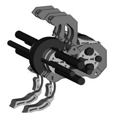
1.2.6 Install the prepared cable or blanking plug in the multiple hinged clamp. Make sure that the raised ridge on the inside of the clamps fits into the groove in the rubber of the branching plug (check this during the installation of both clamps).
