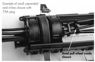
1.3.1 Locate the outside clamps in the closure base by rotating the clamped branching plugs until the square hole (with two lock pins) in the outside clamp is above the raised plastic location post in the outside recess in the closure base. Press the branching plugs into place.
