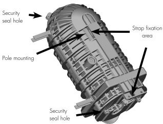
1.3.7 Mounting and security seal positions on the closure(s).
