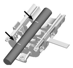
1.1.2 For large and small closures centre the bottom half of the closure around the joint and mark the position of the inner and outside edges of the branching plug recess onto the cables.
