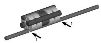
1.1.4 Install the branching plug onto the cable(s) in the appropriate port having removed the blanking rod(s) (see selection table on page 1). **Note**: taping the cables together each side of the plug will help to keep the plug in position (1).
