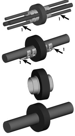
1.2.5 Wrap the length of gel tape around the centre of the branching plug or port reducer. Do not stretch the gel sealing tape during wrapping.
