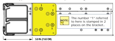
**3.5" Offset Position** To mount bracket at 3.5" position remove screws from holes marked "1" and remount bracket using unmarked holes.
