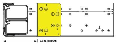
**6" Offset Position** To mount bracket at 6" offset, remove 4 screws from holes marked "1" and rotate bracket 180 degrees. Reinstall 4 screws in holes marked "1".
