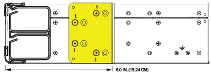
**9" Offset Position** To mount bracket at 9" offset, remove the 4 screws from holes marked "1", rotate bracket 180 degrees, reposition bracket at rearward position, and reinstall 4 screws in holes marked "1".
