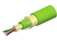
Fiber indoor cable, LazrSPEED® Low Smoke Zero Halogen Riser MPO Trunk with 2.0mm Subunits, 12 fiber, Multimode OM5, Gel-free, Feet jacket marking, Lime green jacket color, B2ca Flame rating
