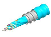
Fiber indoor cable, LazrSPEED® Riser/LSZH rated, MPO Trunk, interlocking aluminum armored, Multimode OM4, 144 fiber multi-unit with 12 fiber subunits, Gel-free, Feet jacket marking, Aqua jacket color, B2ca flame rating
