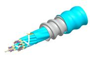
Fiber indoor cable, LazrSPEED® Riser/LSZH rated, MPO Trunk, interlocking aluminum armored, Multimode OM4, 192 fiber multi-unit with 12 fiber subunits, Gel-free, Feet jacket marking, Aqua jacket color, B2ca flame rating
