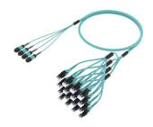
Ultra Low Loss ULL OM4 MPO8 UPC pinned to LC/UPC Uniboot Ruggedized fanout Cable, 32-Fiber, Dual Rated (OFNR/LSZH), 8 fiber PmP 2.0 mm
