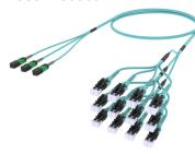
Ultra Low Loss ULL OM4 MPO8 APC non-pinned to LC/UPC Uniboot Ruggedized fanout Cable, 24-Fiber, Dual Rated (OFNR/LSZH), 8 fiber PmP 2.0 mm
