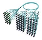
Ultra Low Loss ULL OM4 MPO8 APC non-pinned to LC/UPC Uniboot Ruggedized fanout Cable, 144-Fiber, Plenum, 8 fiber PmP 2.0 mm
