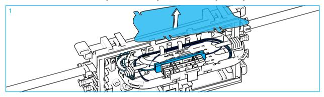
1 Remove the cover of the tray and guide the output of the splitter to the patch panel.
