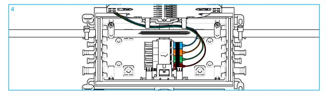
4 Connect the SC connector to its assigned port. A clicking sound is observed when the connector is properly seated. Dress the patch cords under the tabs as shown. All 4 SC connectors installed.
