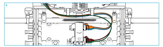
4 Connect the LC connector to its assigned port. A clicking sound is observed when the connector is properly seated. Dress the patch cords under the tabs as shown. All 4 LC connectors installed.
