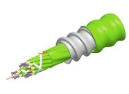
Fiber indoor cable, Plenum MPO Trunk, interlocking aluminum armored with plenum jacket, 48 fiber multi-unit with 16 fiber subunits, Gel-free, OM5 multi-mode, Feet jacket marking, Lime green jacket color
