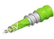
Fiber indoor cable, Riser/LSZH rated, MPO Trunk, interlocking aluminum armored, OM5 mult-mode, 64 fiber, Feet jacket marking, Lime green jacket color, B2ca flame rating
