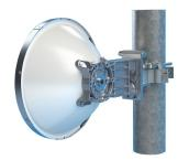
0.3 m | 1 ft ValuLine® High Performance Low Profile Antenna, single-polarized, 12.700–13.250 GHz, OEM custom flange, white antenna, gray radome without flash, standard pack—one-piece reflector
