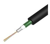
Fiber indoor/outdoor drop cable, LSZH, Gel-filled Central Tube, CST, 2 fiber, Multimode OM4, Meters jacket marking, Black jacket color
