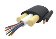
Fiber Hybrid drop cable, LightScope ZWP® Fiber + Tone Wire Outdoor, 4 fiber Arid Core construction, central loose tube, Gel-filled, Singlemode G. 652.D and G.657.A1, Feet jacket marking, Black jacket color, 2000 ft
