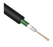
Outside Plant Fiber Optic Cable, HDPE, 8-fiber, Multimode, OM3, loose tube, gel-filled, 1000 m
