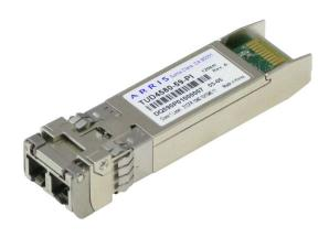
TUD4580 modules feature a very low jitter contribution, resulting in extremely clean, high-quality eye patterns. The module's metal enclosure ensures rugged durability and improves FCC EMI test margins. This emission and ESD control are particularly important in applications with sensitive multiport hubs and switches. The modules, which dissipate less than 2.0 W, are supplied with a duplex LC connector.
