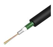
Fiber OSP cable, PE, Gel-filled Central Tube, CST, 8 fiber, Singlemode G. 652.D and G.657.A1, Meters jacket marking, Black jacket color
