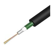
Fiber OSP cable, PE, Gel-filled Central Tube, CST, 24 fiber, Singlemode G. 652.D and G.657.A1, Meters jacket marking, Black jacket color
