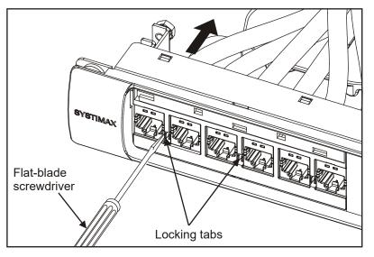
1. Insert a small, flat-blade screwdriver or other small, blunt-end tool in between locking tab and side of outlet as shown to release it. Disengaging one tab will release outlet.
