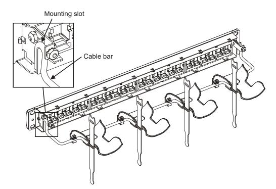
2. Attach cable bar to rear of panel as shown. For 48-port panels, two cable bars are provided.
