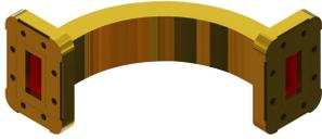
90° E Plane Swept Bend for WR137, 5.85–8.2 GHz, with interface types PDR70 and UDR70, 102 mm x 102 mm, gray
