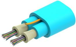
Fiber indoor cable, LazrSPEED® Plenum for MPO Trunks, 48 fiber with 24 fiber subunits, Multimode OM4, Feet jacket marking, Aqua jacket color
