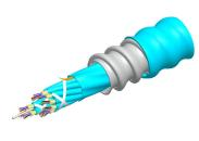
Fiber indoor cable, LazrSPEED® Riser/LSZH rated, MPO Trunk, interlocking aluminum armored, Multimode OM4, 24 fiber with 12 fiber subunits, Gel-free, Feet jacket marking, Aqua jacket color
