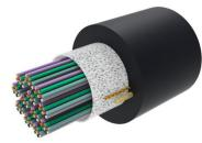
Fiber indoor/outdoor cable, All-Dielectric, LSZH, Gel-Free, Riser Rated, Central Core Rollable Ribbon, 2880 fiber, Singlemode G.657.A2, Feet jacket marking, Black jacket color, Cca flame rating
