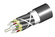
Fiber Indoor/Outdoor cable, LazrSPEED®, Low Smoke Zero Halogen Riser Distribution Cable, 36 fiber multi-unit with 12 fiber subunits, Gelfree, Multimode OM4, Feet jacket marking, Black jacket color, Cca flame rating
