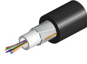
Outdoor Fiber Optic Cable, 12-fiber, singlemode, OS2, PE, loose tube, gelfilled, cut length
