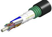
Fiber Optic Cable, Indoor/outdoor Low Smoke Zero Halogen, CPR-only flame rated, Stranded Loose Tube CST Armored Cable
