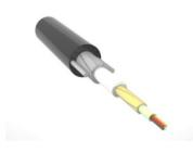
Fiber Drop Cable, Duct and Aerial, FTTH, 4 fibers, Singlemode, G.657.A1, Gel-filled, Feet jacket marking, Black jacket, dual sheathed with indoor element (Dca class for subunit only)
