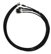
HELIAX® M-LOC Multiport cluster 5 ports SureFlex® cable assembly with Integrated Birdproofing Shell with interface type M-LOC latching male to 4.3-10 male,size 1/4", length 2 meters
