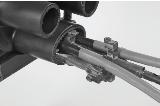
3.2.3 Feed the loop trough the oval port such that the hose clamps are \pm 5 cm in the port.
