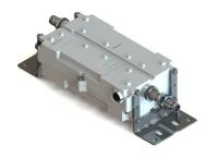
Interference Mitigation Filter for 2600 MHz B7 band with rejection 46dB in 2575-2615 MHz band
