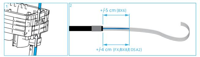
1 Feed the cable through the port. Cutting the cable edge under 45° will help to feed the cables through the RSKG seal. Prepare as per standard practice.
