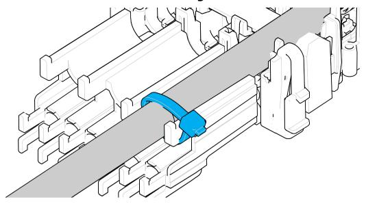
Secure the feeder cables to the external cable guidance bracket using a cable tie.
