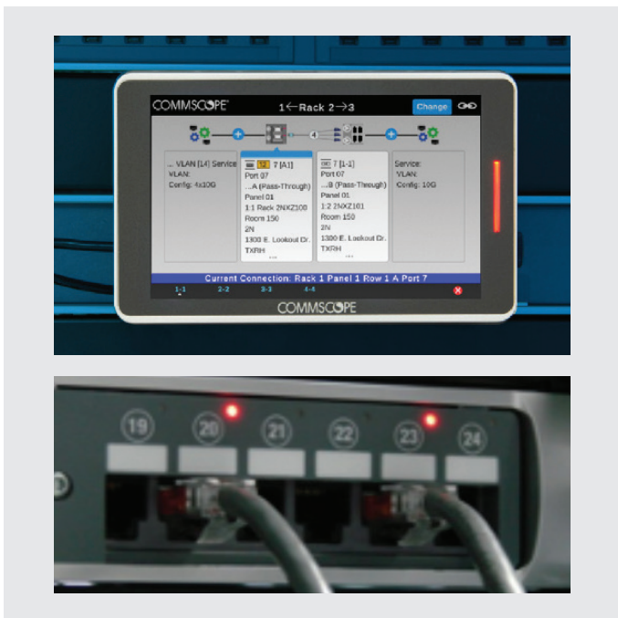
Figure 1: imVision provides on-screen instructions and visual guidance on port connectivity to ensure accurate changes.
