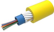
Fiber indoor/outdoor cable, LightScope® ZWP, dry loose tube, 4 fiber, Singlemode G.652.D and G.657.A1, Gel-free, Yellow jacket color, Dca flame rating. Provides Rodent Resistance
