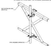
RRU Angle Mount Kit for Angle Sector Frame Members (mounts 1.88 to 3.5in OD pipes to back of 90 degree angles 1.5in to 3in - Pipe not incl)
