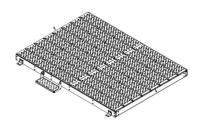
Equipment Platform, 8 ft x 11 ft, base with Pier Connections
