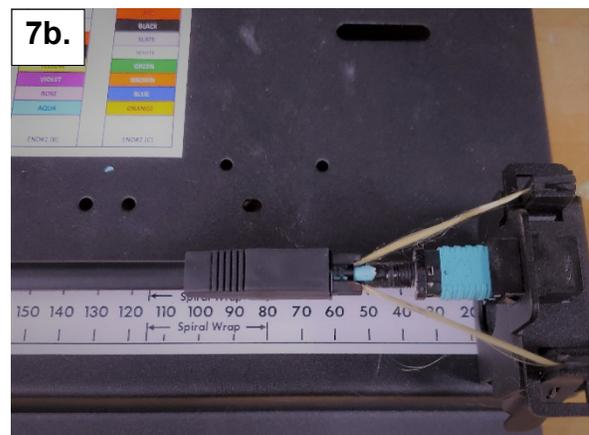
7. a: Trim the jacket up to the slotted edge (dotted line) as shown. Do not trim too short. The jacket should rest in the slotted area of the rear housing.
