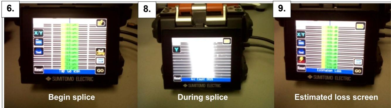
9. After the splice is complete, estimated results will display: green for passing, red for failing. Open the door and remove the assembly from the fiber clamps.
