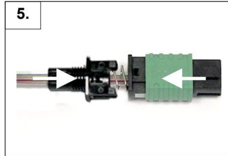
5. Snap outer housing onto the end of the rear housing. Slide the outer housing over the ferrule and spring, snap onto the end of the rear housing.
