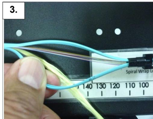
1. Remove the tape or clip holding the cable jacket and the strengthening yarn.
