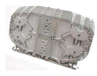
FIST® Splice Sub-assembly kit for GCO2-FC/FD flat closures with 6 slim High Density (HD) element trays, each for holding up to 24 primary coated fibers, with Heat Shrink type splice holder
