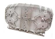
FIST® Splice Sub-assembly kit for GCO2-FC/FD flat closures with 4 slim High Density (HD) element trays, each for holding up to 24 primary coated fibers, with Heat Shrink type splice holder
