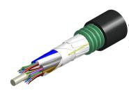
Fiber indoor/outdoor cable, TeraSPEED®, Single Jacket/Single Armor, 90 min Fire Survival, Low Smoke Zero Halogen (LSZH), 12 fiber, Singlemode G.652.D and G.657.A1, Gel-Filled, Stranded Loose Tube, Black jacket color, Meters cable marking
