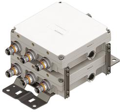
Twin Triplexer 1350-1525//18//21-23-26 MHz, dc smart bypass, with 4.3-10 connectors
